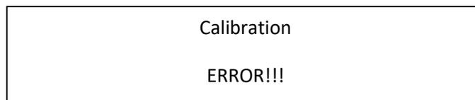
Exit this the menu with the ESC key and Check that the buffer and connections are intact
