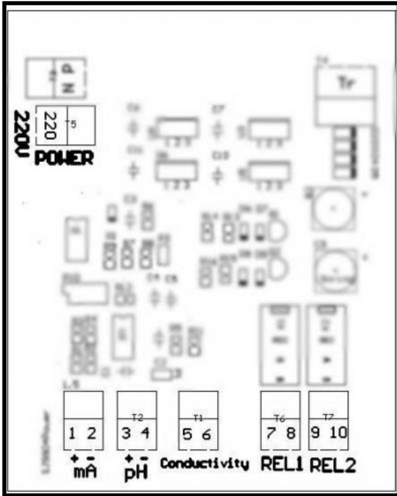
1 and 2- Location of Output connection Fluid(Non-isolated)
