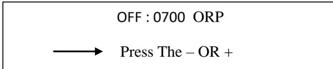
By Using the keys ▼ and ▲, you can select the appropriate ORP value to send the off command, this means that the device by reaches to this ORP value, Issues the command to turn off relay 1. It is best to select the on and off values at appropriate intervals so that the device does not fluctuate (More than a few hundred ORP). After selecting the appropriate number, press the E key once to save the information.
